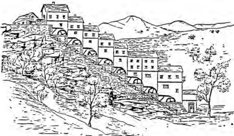
19. Barbegal: reconstruction of multiple mill (Benoît)
